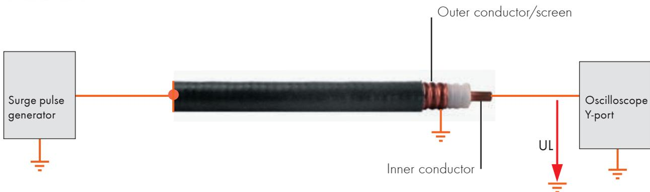
Such a surge suppressor is not only required due to the leftover residual pulse of the gas discharge tube lightning EMP protector, but also due to magnetic coupling into the possible loop which the antenna cable length between the lightning EMP protector and the equipment is part of (within zone LPZ 1). This is illustrated by the following:
